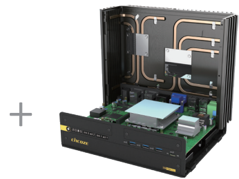
Independent cooling for CPU & GPU
